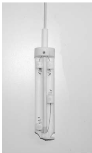
Fig. 6 Thermal conductivity cell for measurement of the thermal properties of electrically conducting fluids
